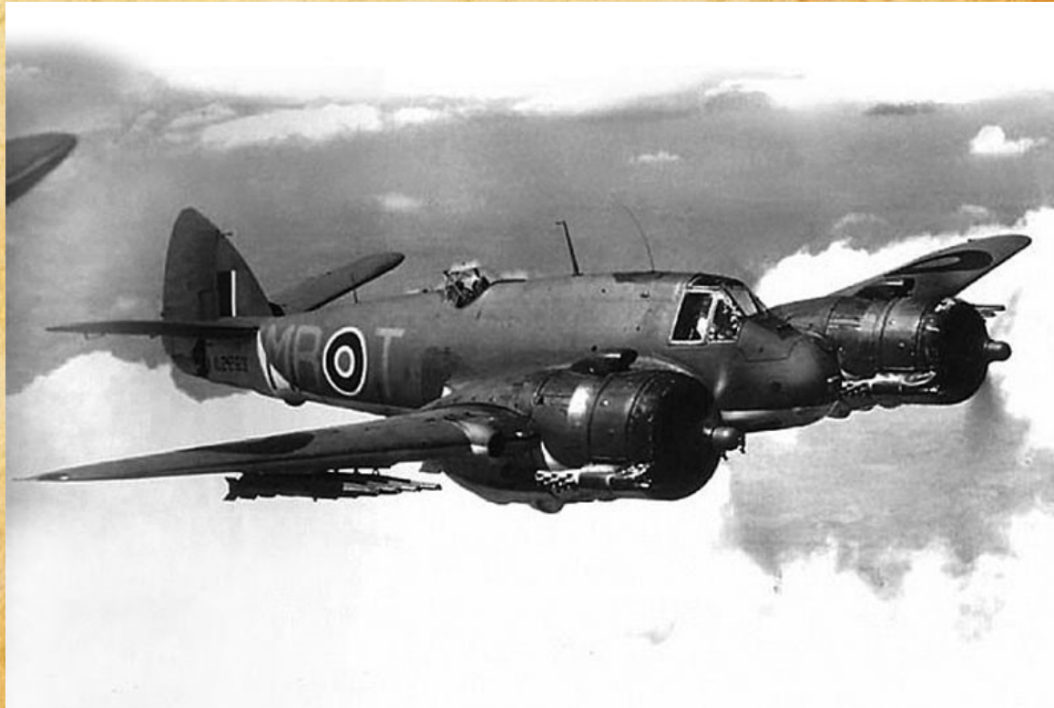
Typical view of a Beaufighter aircraft equipped with rockets. Source: www.militaryfactory.com
